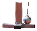
Suspension to check the hammer's length
