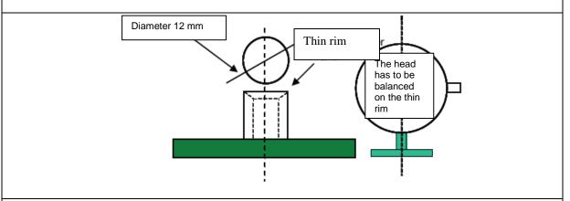
To check the hammer's length, place the hammer with its handle on the suspension (see marking). The head must not lie on the certification unit's foot. If the head is freely movable the hammer is legal.
